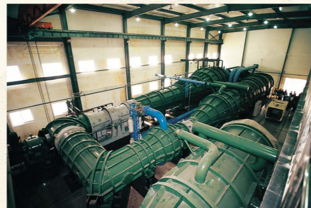
NF-6增压连续式高速翼型风洞 (2004.9)
